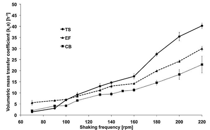
**Fig. 1.** Comparison of  $k_{L}a$  as a function of shaking frequency in OSRs. The  $k_{L}a$  was measured with a static method. The TubeSpin® bioreactor 600 (TS), 1-L Erlenmeyer flask (EF), and 1-L cylindrical glass bottle (CB) were filled with 300 mL of UHP deionized water at 37 °C and orbitally shaken at various shaking frequencies. Each experiment was performed in duplicate.
