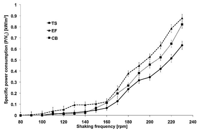
**Fig. 4.** Comparison of specific power consumption as a function of shaking frequency in OSRs. The TubeSpin® bioreactor 600 (TS), 1-L Erlenmeyer shake flask (EF), and 1-L cylindrical glass bottle (CB) were filled with 300 mL of UHP deionized water at room temperature and orbitally shaken at various shaking frequencies. Each value represents the average of six vessels.
